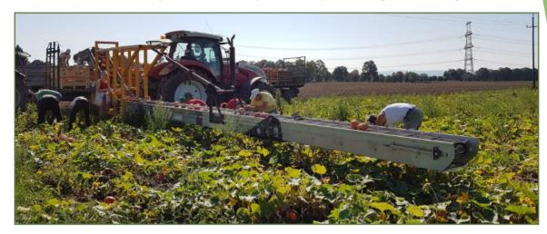
This heavy duty belt brings the crops carefully to an alongside driving trailer without dropping the product. The belt has a swan neck, is hydraulic driven and is adjustable in speed. The belt is available in working widths of 7m up to 11m, with a standard belt width of 40cm. The conveying and discharge height are hydraulically adjustable.
