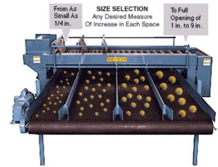
UNEQUALLED ACCURACY - No other diameter grader come close, because of continuous product rotation and individually-driven heavy-duty rollers which maintain precise separation.
